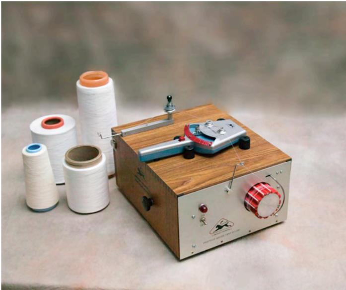
**Friction Meter and Portable Drive Unit LH-603A**
